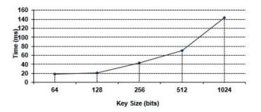
Figure 2. Timing curve for RSA-encryption
