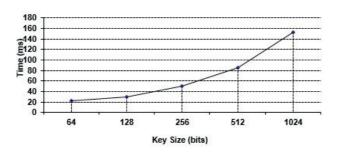
Figure 3. Timing curve for RSA-decryption
